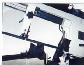
Hydraulic saw arm lifting system for RF-250NA & RF-250NAA
