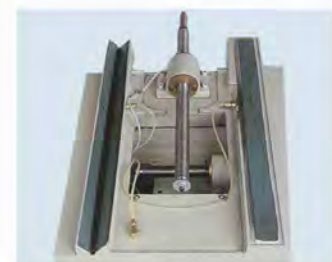
◆ The VEE & FLAT slide ways coated with turcite-B. Plus hand scrapped
